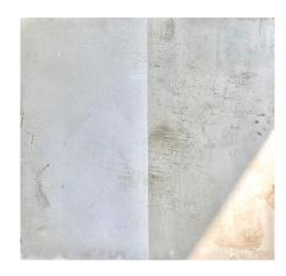
The concrete is allowed to dry for 72 hours to ensure full curing before subjecting to heavy contamination.
