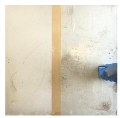
A single, even coat of Graffiti Resist is applied to the right of the clean surface with a pad. This will ensure even distribution of product for testing purposes. (Other methods of application are suitable such as roller, brush or airless spray)
