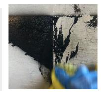
Graffiti Resist demonstrated excellent resistance against spray paint, allowing the treated half of the concrete to return to its original condition after cleaning.
