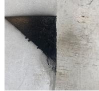
A generous coat of solvent based spray paint is applied to the half treated test piece.
