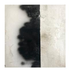
The treated concrete performed very well, the spray paint was wiped away with a cloth and light cleaner. Power washing will remove graffiti using just water.
